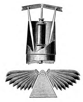
The boiler is constructed with a number of small tubes to give a large heating surface with small amount of weight, as well as requiring a very small amount of water; and the heat is obtained by burning vaporized hydrocarbon combined with a hot-air blast. The exhaust steam is condensed in a hollow tail, thus saving weight in the quantity of water required. This tail also serves the purpose of a supporting surface (*i. e.* aëroplane).
